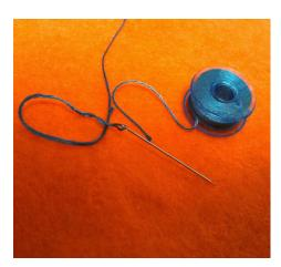
Using conductive thread is easy. I only sew with one line of thread at a time. But with "regular thread" I normally "double" the thread on the needle for strength.
