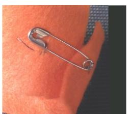
9. When you connect the safety pin to the lines of thread you made in step 7, you complete the circuit. Put on your bracelet and shine!
